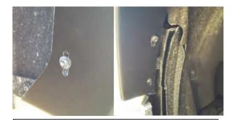
**STEP 5:** Reinstall the remaining 5.5mm bolt and two 7mm bolts.
