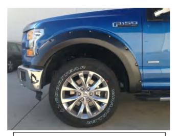
**STEP 6:** Repeat installation method for other side. Double check the front Fender Flares to make sure all bolts are tight and clips are securely fastened. Your installation is now complete. Do not use abrasive cleaners.
