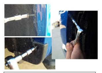
**STEP 4:** Insert four (4) of the .9mm lever retaining clips (two (2) per side) into the Fender Flare. Make sure the tab in the clip securely attaches in the slot on the Fender Flare. Secure with five (5) bolts removed in Step 6.
